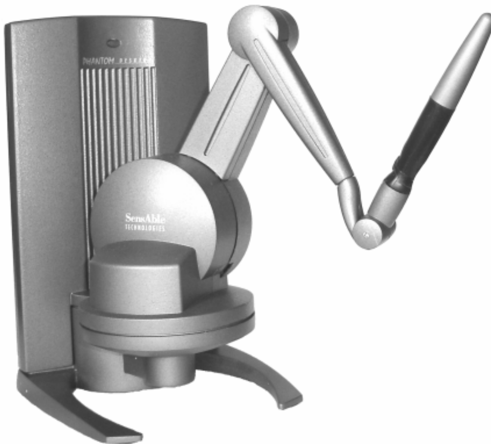
Fig. 10: SensAble Phantom Device – An interface to simulate haptic interaction.
